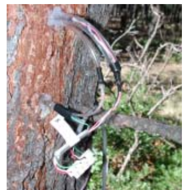
Granier sap flow sensor in a Ponderosa
