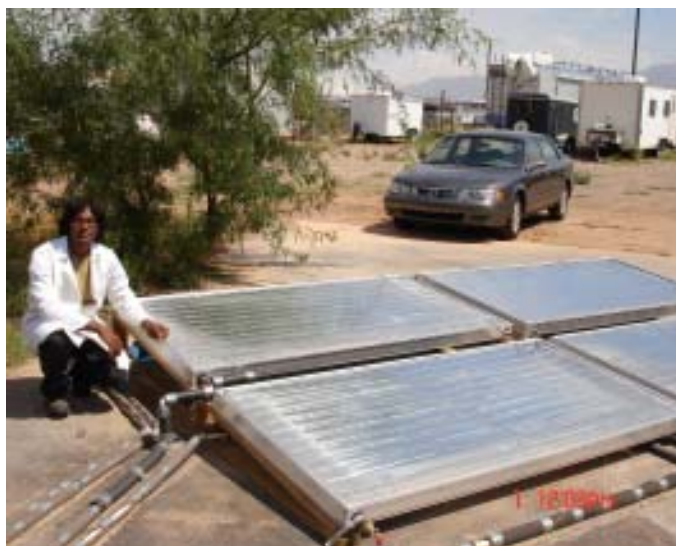
Prajwal Vikram, a graduate student pursuing a master's degree in chemical engineering at New Mexico State University, examines the solar collectors for a solar-powered desalination project.
