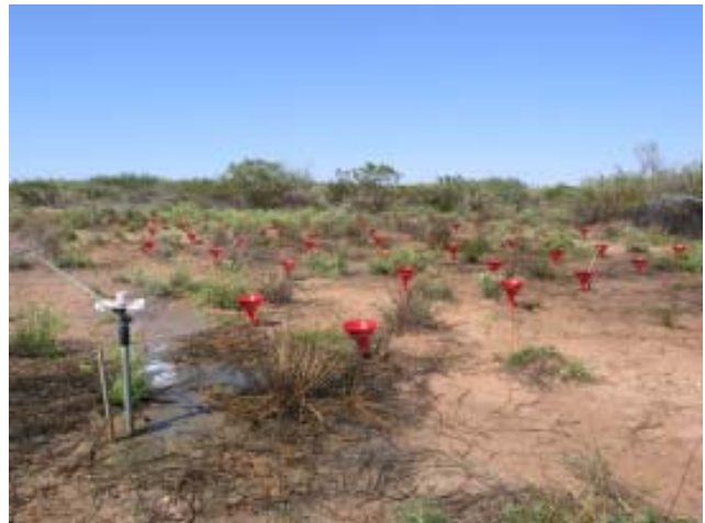
Field layout of the funnels for 4-point sprinkler distribution uniformity assessment for Chihuahuan Desert soils at West Mesa irrigated with industrial effluent (American Society of Agricultural Engineers standard #S330.1, 1993)
