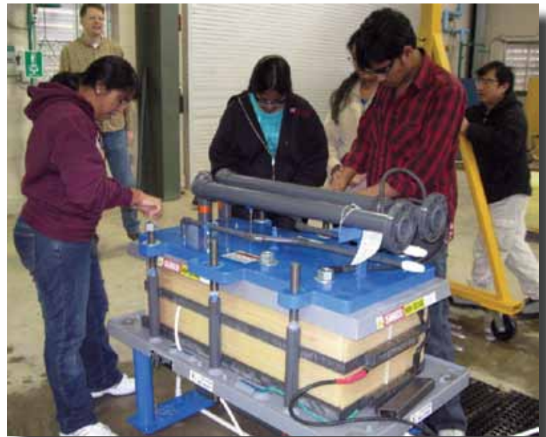
NMSU graduate students work with a hybrid experimental Electrodialysis Reversal (EDR) unit at BGNDRF. The unit is designed so various inputs and components in the desalination process can be varied and results measured. (Photo by Karen Mikel)
